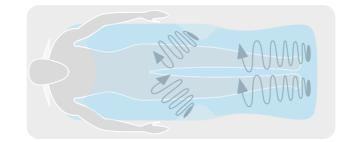
The authentic Jacuzzi® hydromassage has jets inclined at 30°, which can be positioned in any direction.
